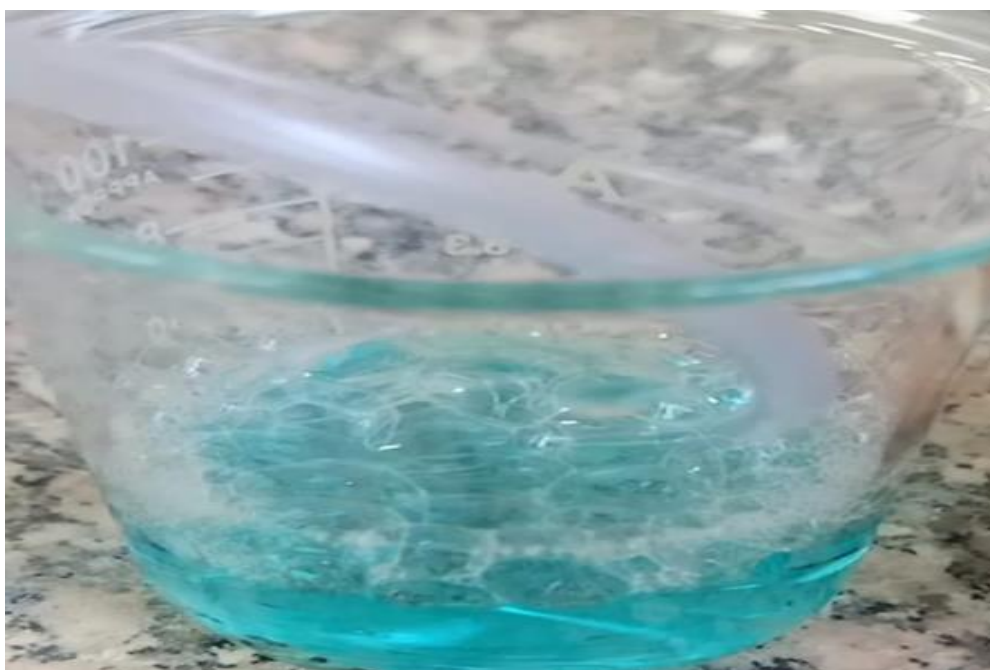
Figure (2): Bubbles observed when the gas produced from the cannula was exposed to the soap solution.
