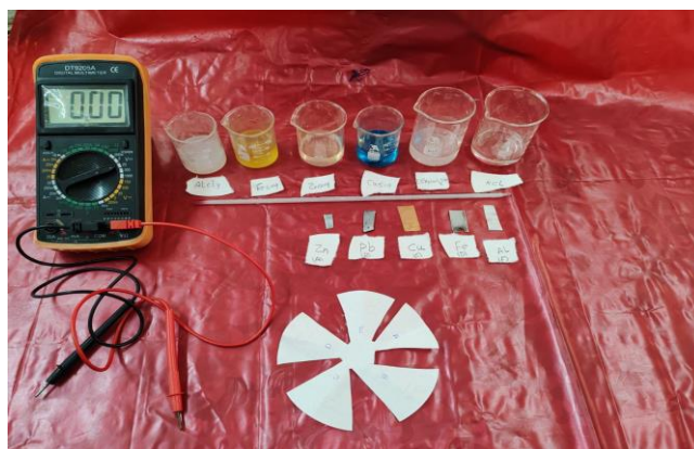
Figure (1): Equipment and materials needed for the fabrication of galvanic cells.
