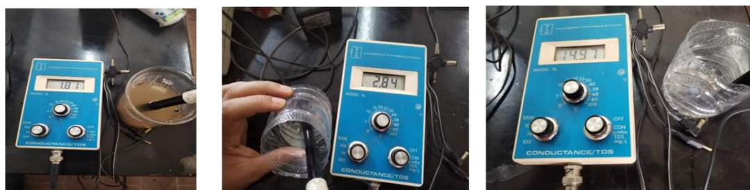
Fig 8: Conductance measurements of polluted and purified water samples
