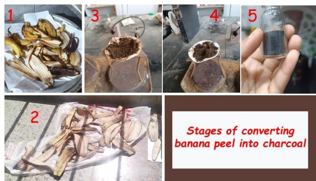
Fig 4: Showed the stages of converting the banana peel into charcoal.
